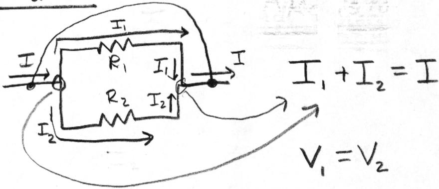
$$\frac{1}{R_{eq}} = \frac{1}{R_1} + \frac{1}{R_2} \dots$$
