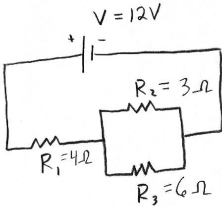
a) Find equivalent resistance of circuit.
