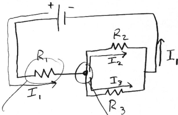
Total current must pass through  $R_1$
