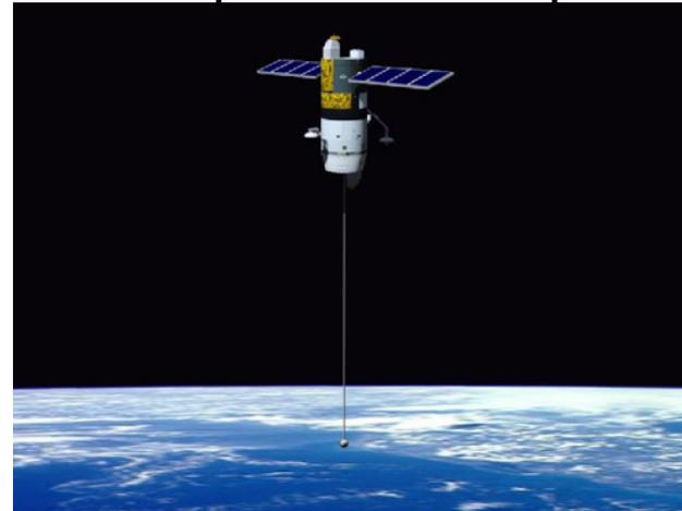
In 1996, NASA conducted an experiment with a 20,000-meter conducting tether. When the tether was fully deployed during this test, the orbiting tether generated a potential of 3,500 volts. This conducting single-line tether was severed after five hours of deployment. It is believed that the failure was caused by an electric arc generated by the conductive tether's movement through the Earth's magnetic field.
