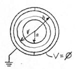
Two conducting hemispherical shells of inner radius b are then brought up and, without contacting the solid sphere are connected to form a spherical shell surrounding and concentric with the solid sphere as shown below The outer shell is then grounded.
