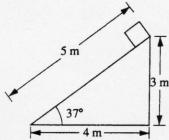
15. A plane 5 meters in length is inclined at an angle of 37°, as shown above. A block of weight 20 Newtons is placed at the top of the plane and allowed to slide down. The work done on the block by the gravitational force during the 5-meter slide down the plane is most nearly
